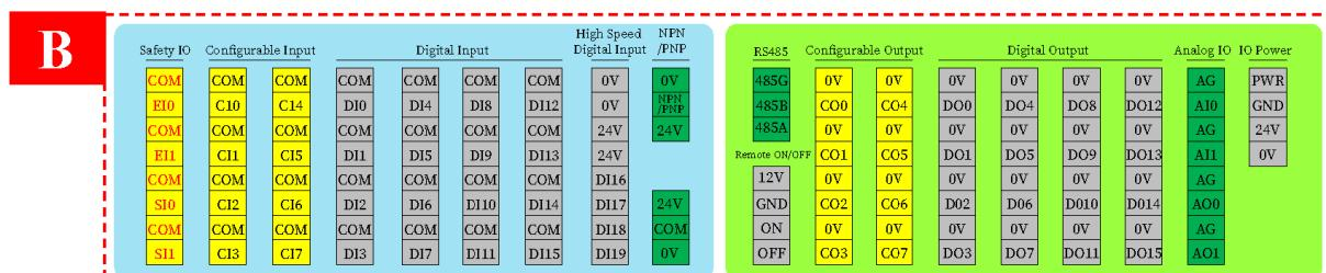
The diagram shows the layout of the Control Cabinet Internal Electrical Interface B Area. It includes several connection ports and their corresponding functions:
